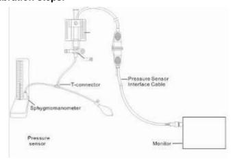
Figure 13 10 IBP pressure calibration connection diagram
