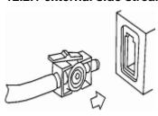
connection between sanpling tube and CO2 side stream
