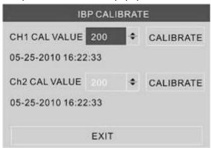
Figure 13 9 IBP pressure calibration menu
